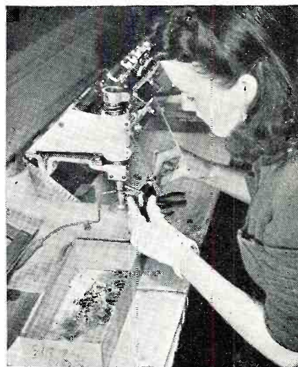
Completing the "mount" or inner structure of a 25-watt transmitting tube.
