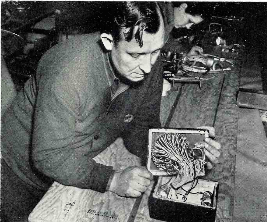
Making final check on the special MULTIPOINT SWITCH for use on wing-electric cable assembly. Accuracy is necessary in its assembly.
