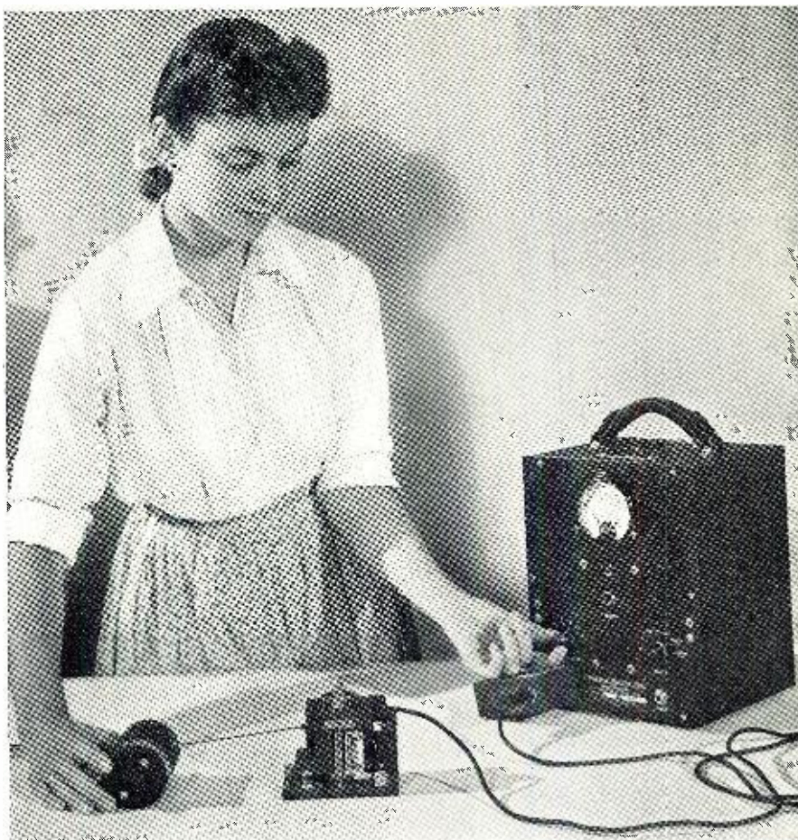
Operating a portable vibration-velocity meter to measure the vibration of bodies in any direction.
