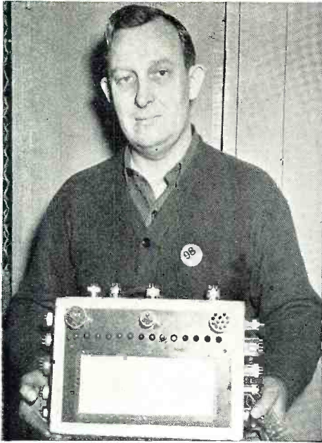
An elaborate tester which checks 72 circuits with one turn of the switch.
