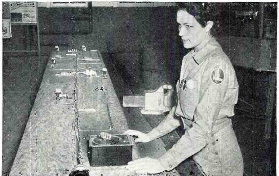
Operator about to test a wing-electric cable assembly. Proper equipment and jigs have reduced operation time considerably.
